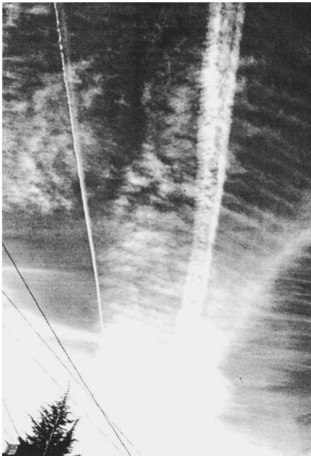
Fig. 3 Condensation wakes shed by three aircraft at different times illustrating how vortex wakes age.
